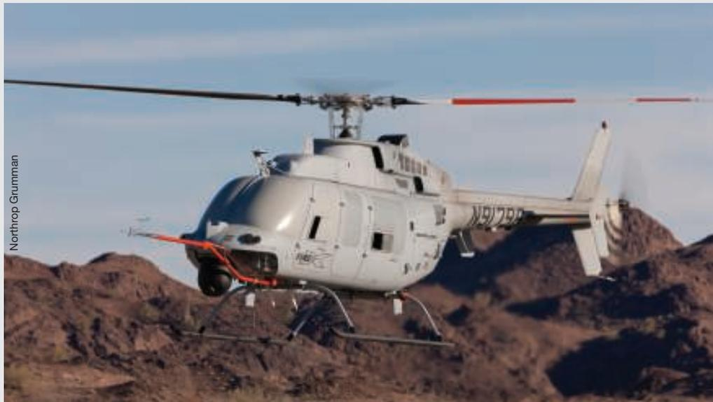
The upgraded MQ-8C Fire Scout will use a Bell 407 airframe and Rolls-Royce 250-C47B dual-FADEC engine.
