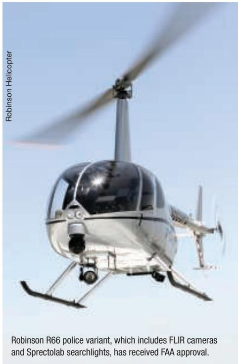
Robinson R66 police variant, which includes FLIR cameras and Spectrolab searchlights, has received FAA approval.
