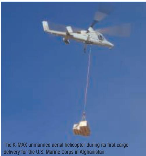
The K-MAX unmanned aerial helicopter during its first cargo delivery for the U.S. Marine Corps in Afghanistan.
