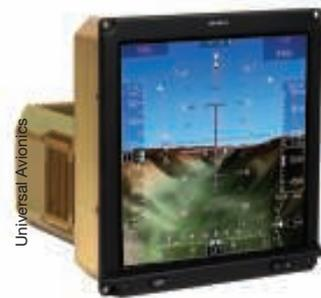
Universal Avionics' flat panel EFI-890H display designed for helicopters.
