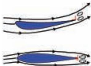
A Gurney Flap "bends" the airflow around a surface in such a way that the surface acts as if it were a different size or shape.
